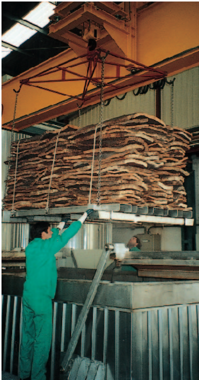
• Natural cork planks are loaded into a hopper at Ponte de Sôr where they are boiled for one hour to remove TCA and other volatile organic compounds.
