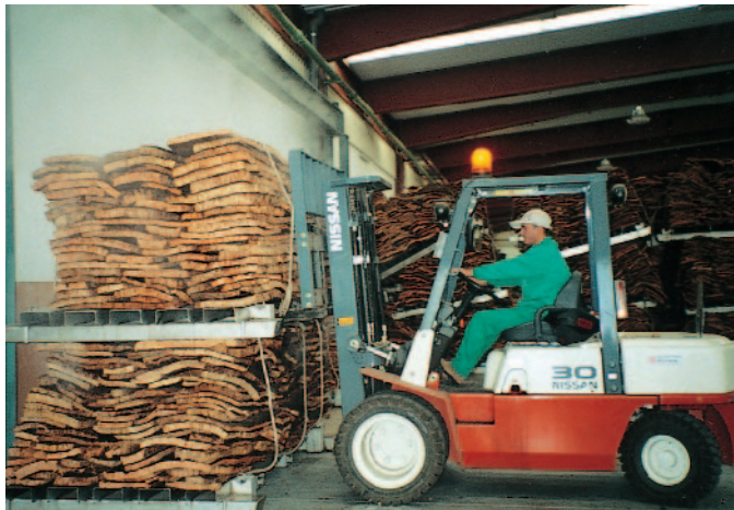
• Still steaming, cork planks are removed from the new boiling system at Ponte de Sôr.
