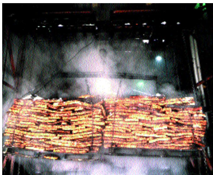
Cork planks are boiled at 100°C
