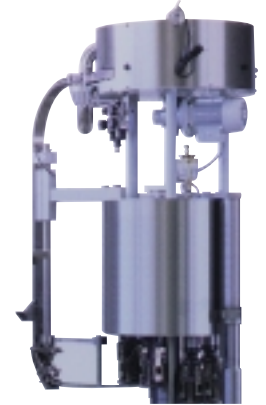
• Multi-head capper for aluminium screw caps
